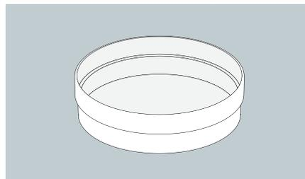
Always use a fresh AQUALAB sample cup and only fill samples half full. **Do not overfill.**
