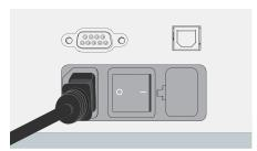
Connect the power cord to rear panel. Then flip the power switch to the On position indicated by an "I".
